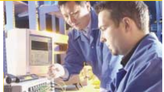
EXFO's IQS-12008 All-Band Component Analyzer performs IL, ORL and PDL measurements over a wavelength range of nearly 400 nm.
